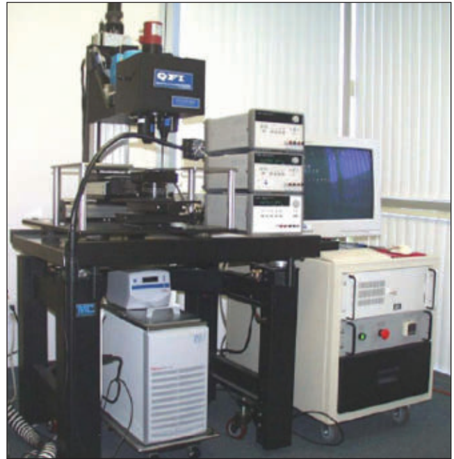
▲ Fig. 2 Infrared camera used to characterize the temperature rise of a package device.
