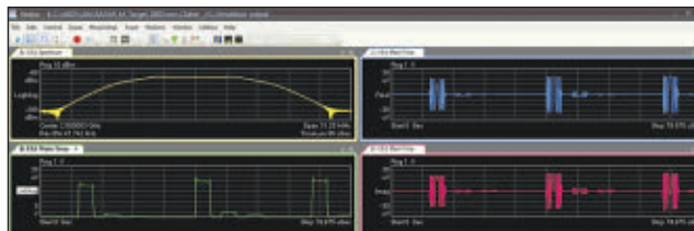
▲ Fig. 3 Generated radar test signals: received spectrum (yellow); and radar target returns with clutter, displayed as amplitude (green), real part (blue) and imaginary part (red).
